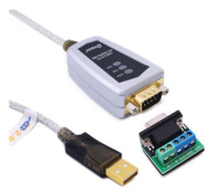
NMEA 0183 communication protocol was designed to run over the RS422 serial interface, which can support a single talker and up to 10 listeners and data rates as high as 10 mbit/sec. RS422 converters in boats are typically used to get or send data to your instruments. You can find USB converters or some Raspberry Pi HATs to connect to the GPIO header.
