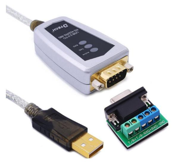
There are normally 4 or 5 connections: TX+, TX-, RX+, RX-, GND.
